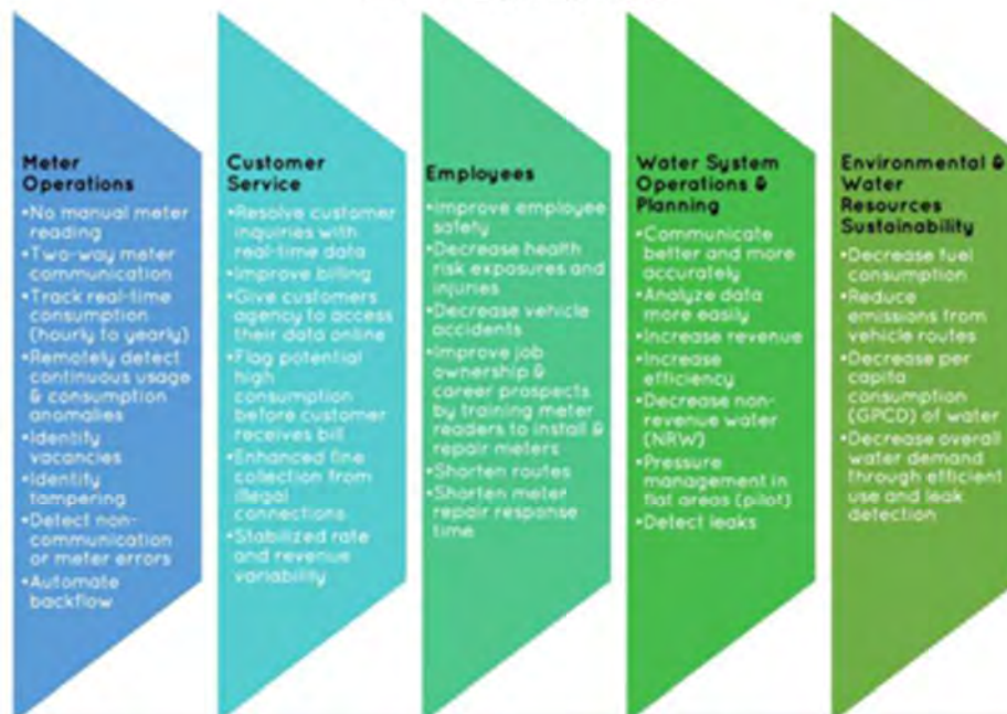
Figure 23: Benefits to the water company of switching to advanced metering infrastructure (AMI) from conventional or drive-by advanced meter reading open (AMR) meters.
