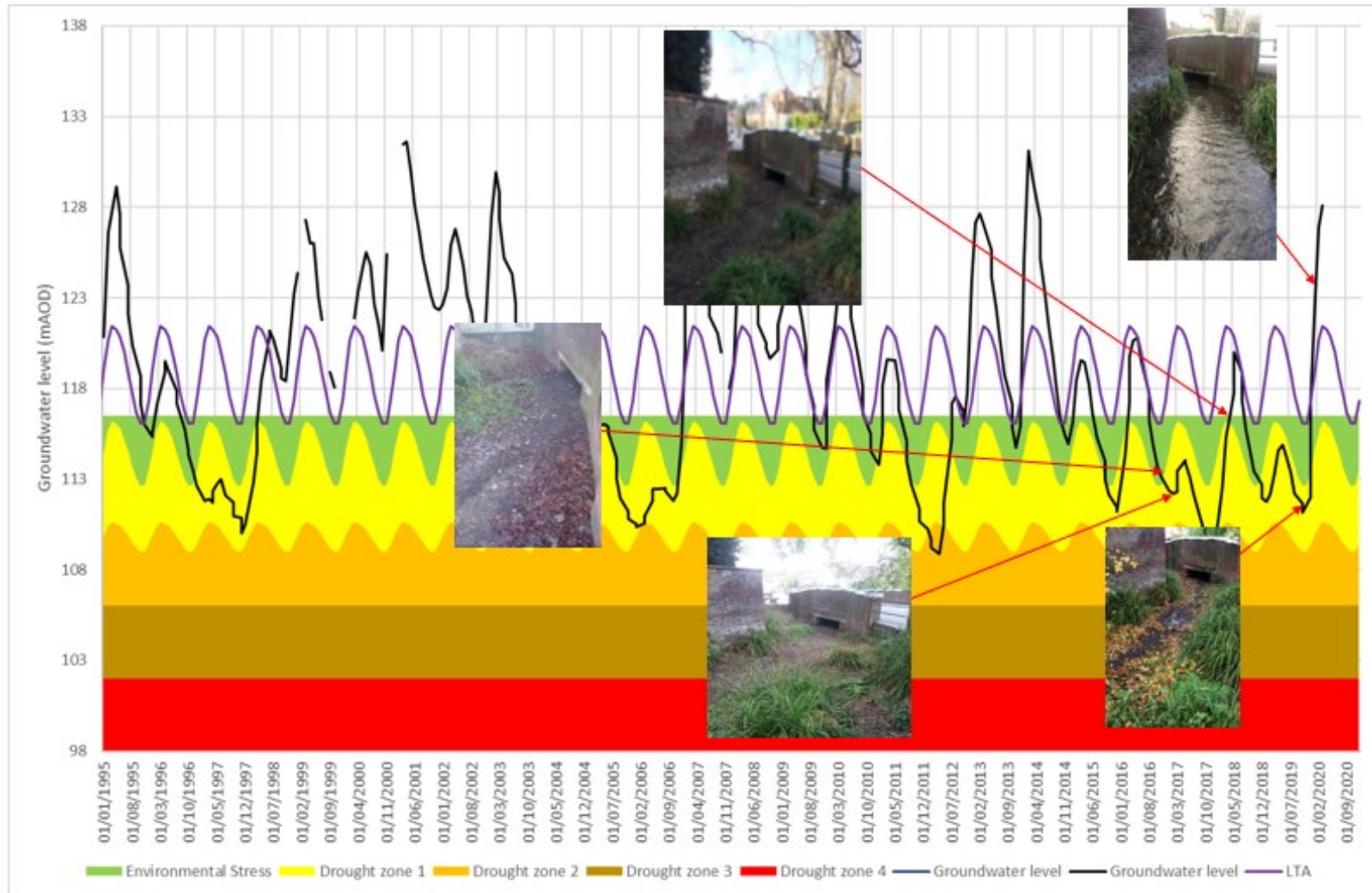
Figure 30: Pictures of the Chess upstream of the Queens Head pub under different hydrological conditions (based on Ashley Green key well)
