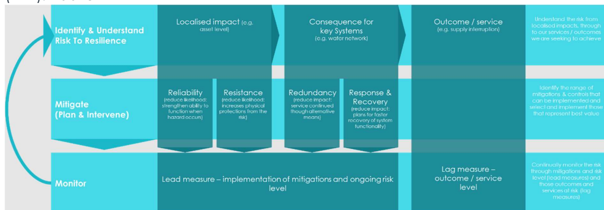
Figure 1, optioneering is undertaken across the '4Rs' (redundancy, response/recovery, resistance, and reliability), to identify the optimal mitigations, supported by assessment using ART, which will continually monitor resilience level post-investment.
